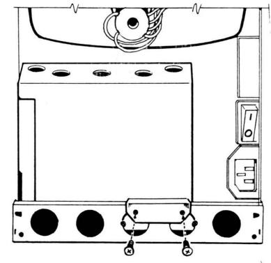
Using three 1/4" screws, fix the clamping plate to the right angle mounting plate as shown. This should clamp the floppy drive housing between the plates.
