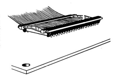
Flip the HyperDrive logic board over aligning with the plastic standoffs over the holes in the Macintosh logic board. It should fit around the keyboard connector.
