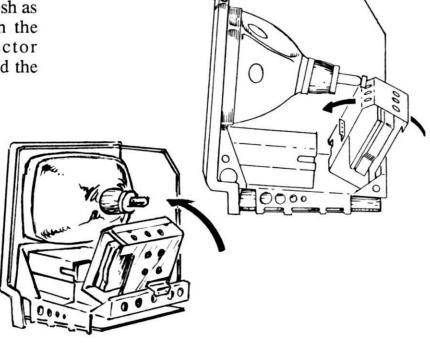
Be sure that the right angle mounting plate goes under the floppy disk housing. This should bring the rear mounting plate on the hard disk housing flush with the outside of the Macintosh chassis. The three screw holes in the right angle mounting plate should not be hidden by the floppy disk housing.
