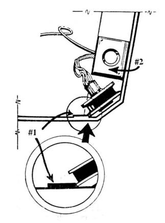
Now mount the controller box by unpeeling the double-sided tape and placing it next to the fan, #2 in the illustration.
