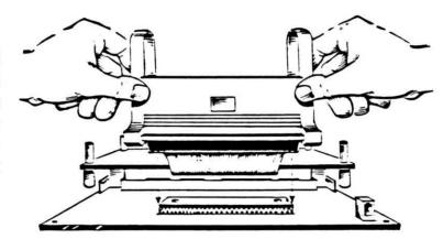
Slip one side of the clip tightly against and under one side of the 68000. Now rock the other side of the clip into position against and under the other side of the 68000 as shown.
