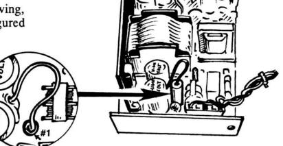
If it is connected at #2 in the drawing, then this power supply is configured for 220V power systems.
