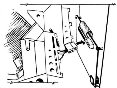
The board assembly will not slide into position like a normal Mac board.
