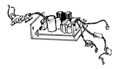
On this power supply the line filter has been incorporated onto the power supply board and a ground wire has been added to the AC power cable.
