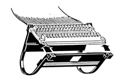
Lay the HyperDrive logic board upside down on the Macintosh logic board as shown.
