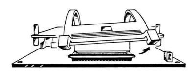
Test by prying under the metal ends of the clip with your fingers as shown. If it comes off, repeat the process of clipping to the 68000.
